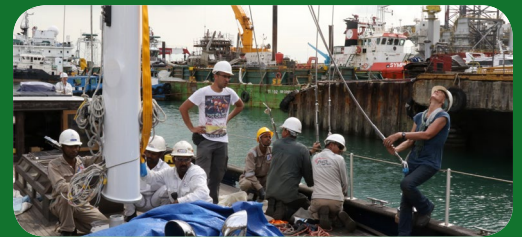
Working with ASL Shipyard to install the masts
