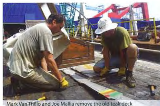
Mark Van Thillo and Joe Mallia remove the old teak deck
